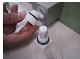
Interfacial trough – Oil/water Trough with electrode in the subphase
